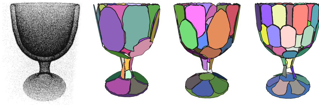
Figure 1: Multiscale Planar Abstraction. Left: Input point cloud of a goblet with outliers and noise. Mid to Right: Planar abstraction with varying fitting tolerance from coarse to fine: 1%, 0.5% and 0.25% of bounding box diagonal.
