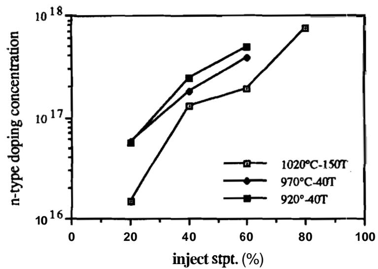
Figure 4.11 Phosphorus concentration determined by C-V measurements vs. dopant set point at various growth conditions.
