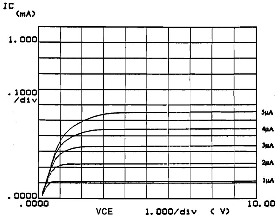
Figure 4.14  $I_C$  versus  $V_{CE}$  characteristics for a representative bipolar transistor fabricated in 970°C-40T SEG.
