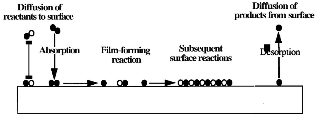
Figure 2.1 Schematic of CVD reaction steps [15].
