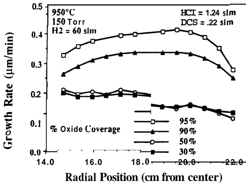
Figure 2.11 Masking oxide area dependence of growth [63].
