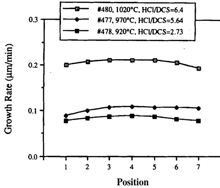
Figure 4.3 (a) Selective epitaxy growth rate profiles on oxide-patterned wafers at 150 Torr and various temperatures.
