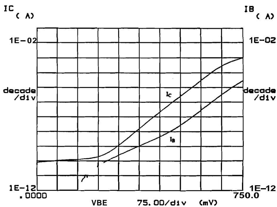
Figure 4.15 (b) Measured  $I_B$  and  $I_C$  versus  $V_{BE}$  characteristics for a representative bipolar transistor fabricated in silicon substrate.
