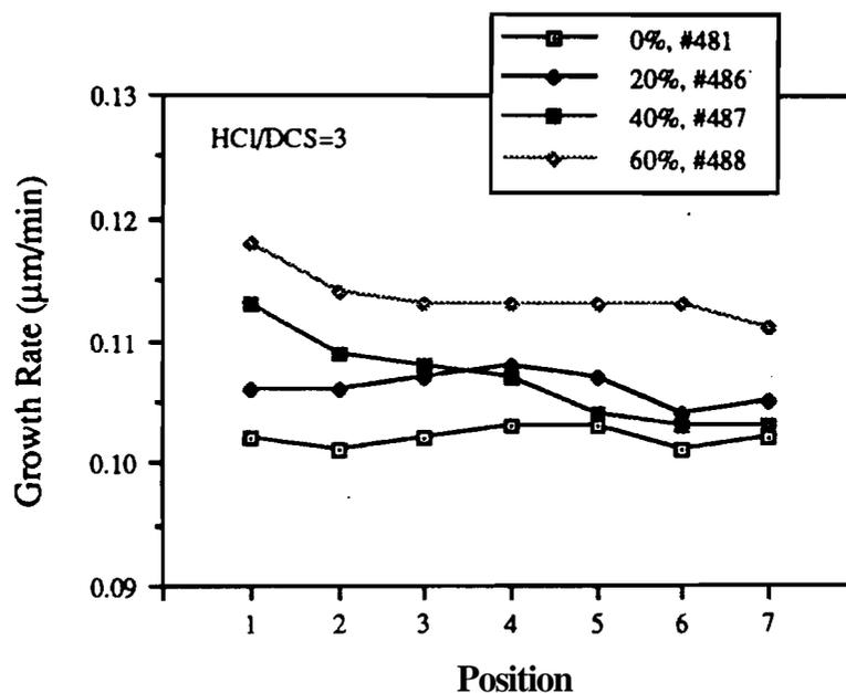
Figure 4.6 (c) Selective epitaxy growth rate profiles on oxide-patterned wafers at 970°C, 40T, and various PH<sub>3</sub> dopant set points.
