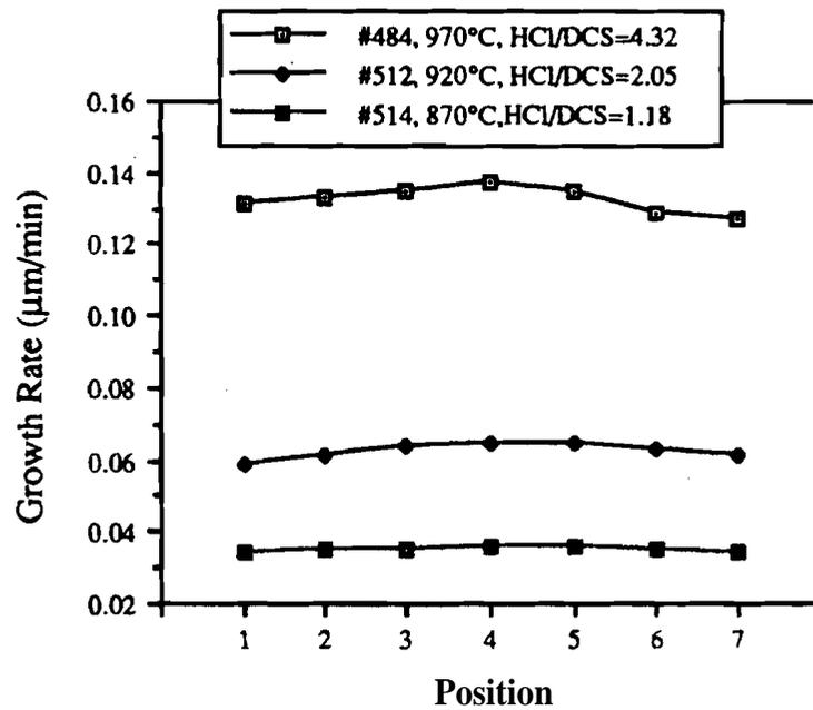
Figure 4.3 (b) Selective epitaxy growth rate profiles on oxide-patterned wafers at 95 Torr and various temperatures.
