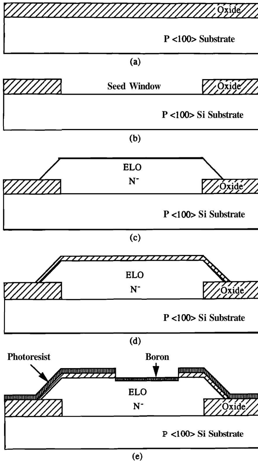
Figure 3.5 Test ELO BJT fabrication process flow.
