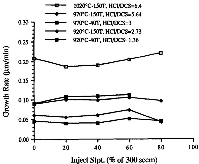
Figure 4.5 Silicon selective epitaxy growth rates vs.  $\text{H}_3$  dopant set points at various deposition conditions.
