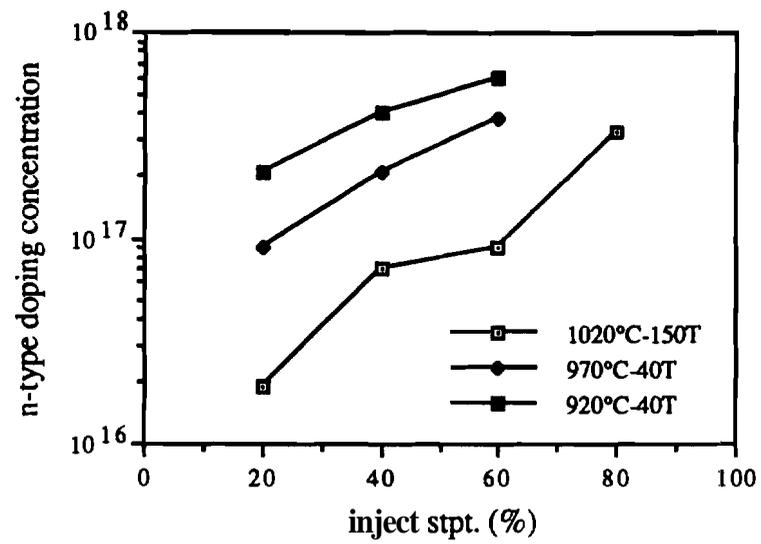
Figure 4.10 Phosphorus concentration determined by resistors vs. dopant set point at various growth conditions.
