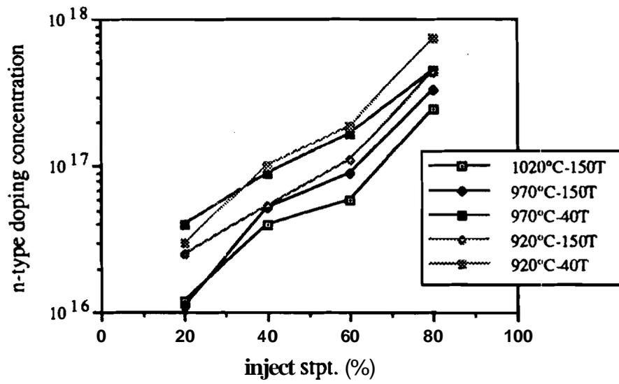
Figure 4.7 Phosphorus concentration determined by four point probe measurements vs. dopant set point at various growth conditions.
