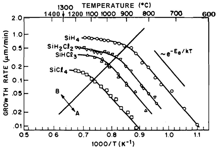
Figure 2.3 Temperature dependence of growth rates for various silicon gas sources [17].
