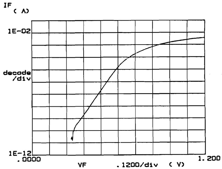
Figure 4.13 Forward bias I-V plot of a representative emitter-base SEG diode.
