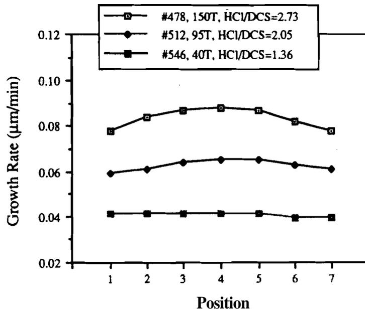
Figure 4.4 (b) Selective epitaxy growth rate profiles on oxide-patterned wafers at 920°C and various pressures.
