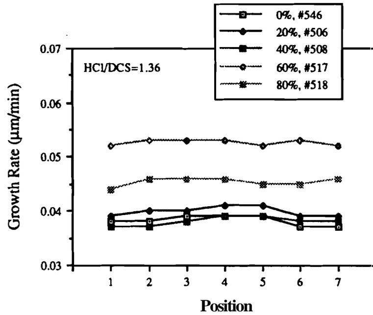
Figure 4.6 (e) Selective epitaxy growth rate profiles on oxide-patterned wafers at 920°C, 40T, and various PH<sub>3</sub> dopant set points.
