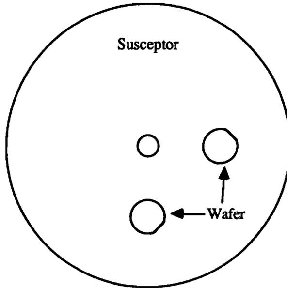
Figure 4.1 Wafer locations on the susceptor.
