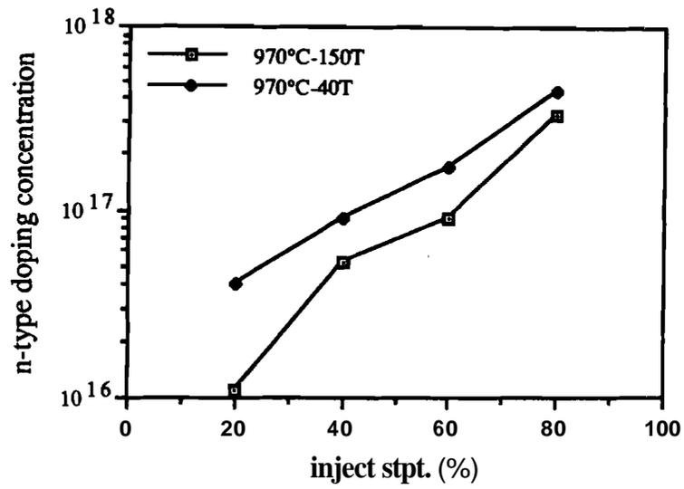
Figure 4.8 (a) Phosphorus concentration vs. dopant set point at 970°C as determined by four point probe measurements.
