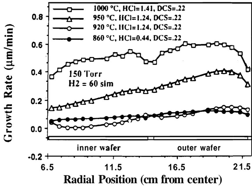
Figure 2.10 Growth rate profile on patterned wafers at different temperatures [63].
