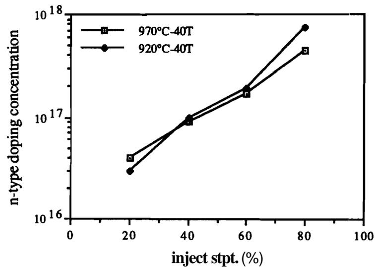
Figure 4.8 (d) Phosphorus concentration vs. dopant set point at 40 torr as determined by four point probe measurements.
