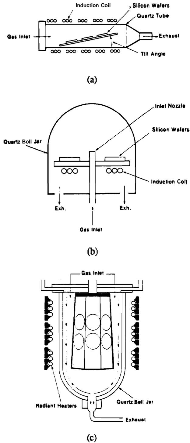
Figure 2.5 (a) Horizontal, (b) pancake, and (c) barrel reactors commonly used for vapor-phase silicon epitaxy [30].
