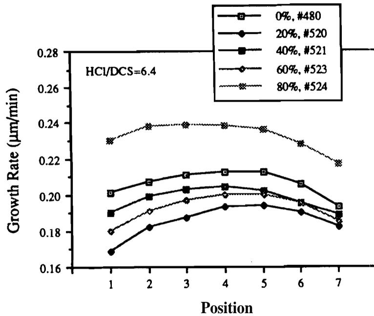
Figure 4.4 (a) Selective epitaxy growth rate profiles on oxide-patterned wafers at 1020°C, 150T, and various PH<sub>3</sub> dopant set points.
