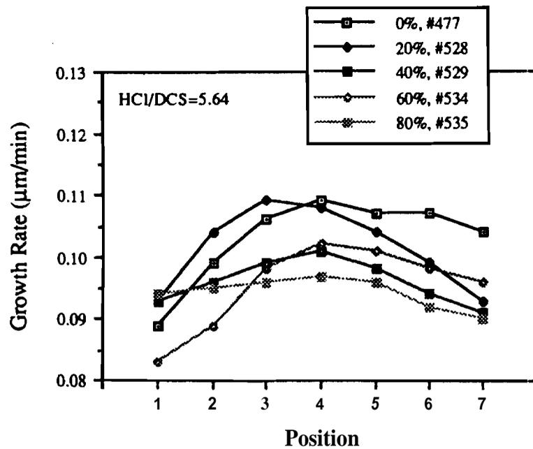
Figure 4.6 (b) Selective epitaxy growth rate profiles on oxide-patterned wafers at 970°C, 150T, and various PH<sub>3</sub> dopant set points.
