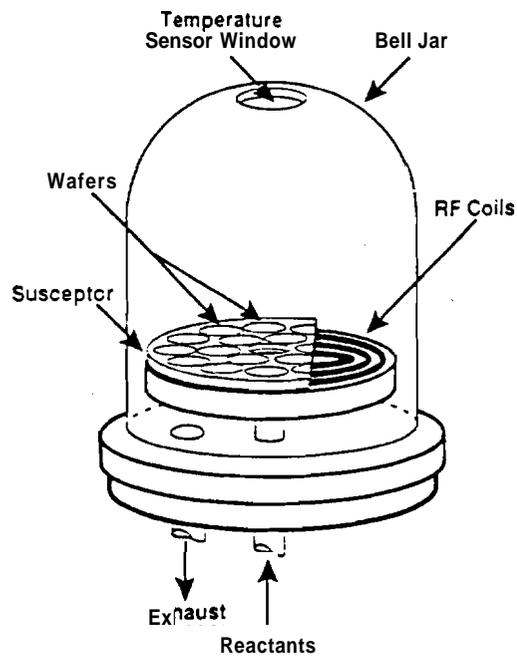
Figure 3.2 Schematic diagram of an induction heated pancake reactor [26].
