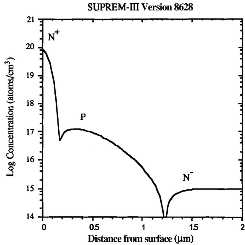
Figure 3.4 SUPREM III simulated plot of net chemical impurity concentration versus depth into the structure for the test device process.
