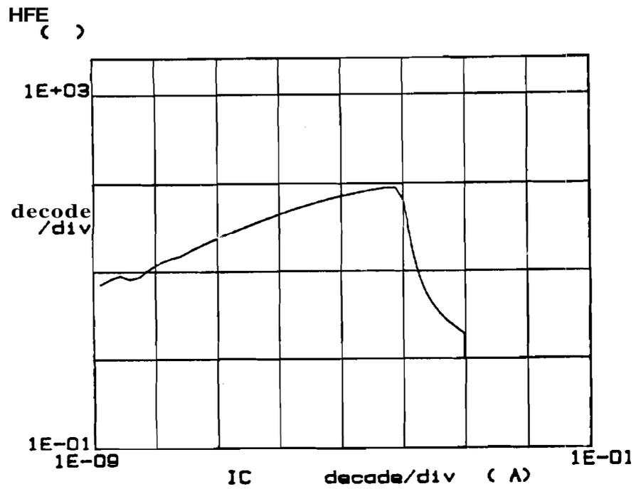
**Figure 4.16 (a)** Measured current gain ( $\beta$ ) versus collector current ( $I_C$ ) characteristics for a representative bipolar transistor fabricated in 970°C-40T SEG.
