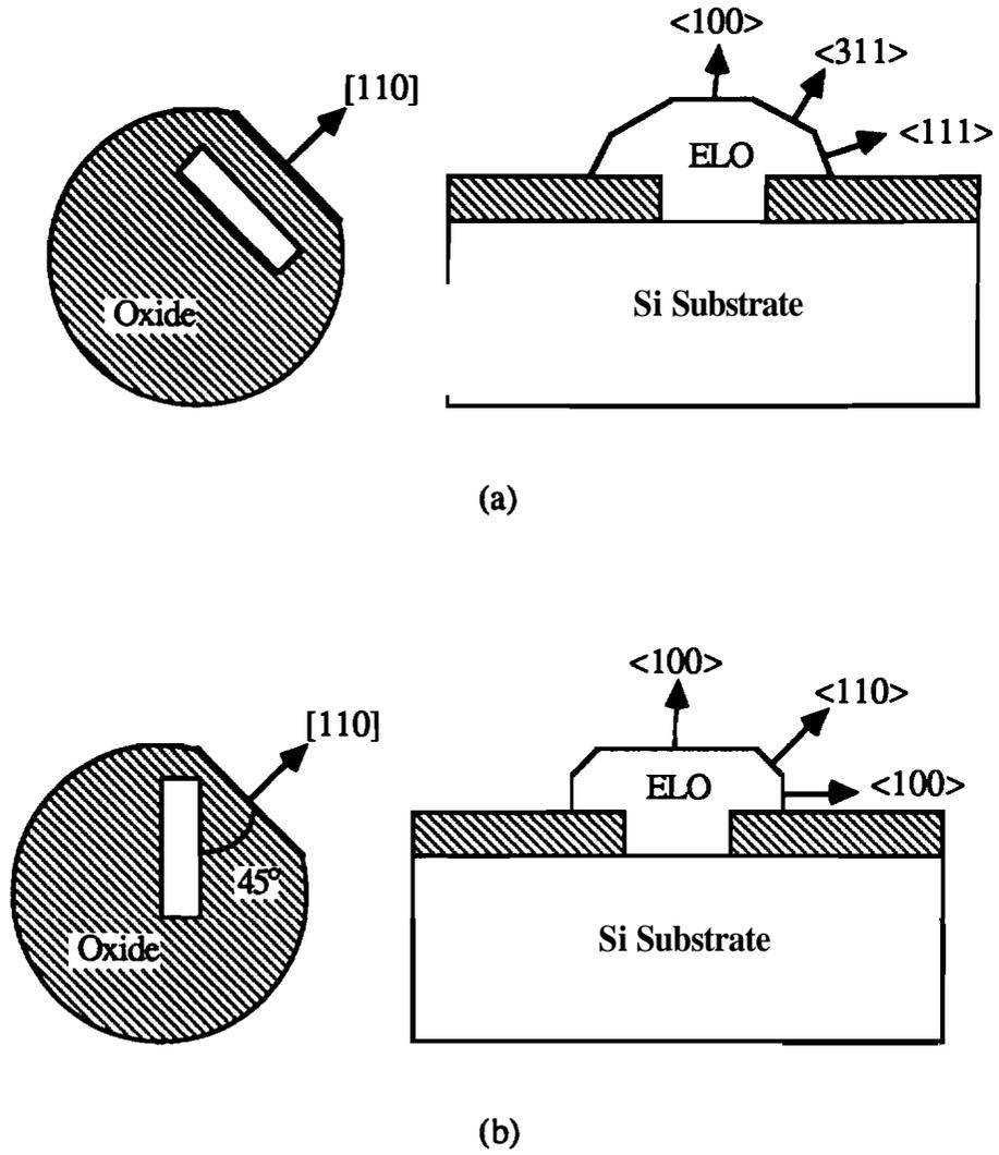
Figure 2.9 ELO facets : (a) Seed window is along  $\langle 110 \rangle$  directions. (b) Seed window is along  $\langle 100 \rangle$  directions [62].
