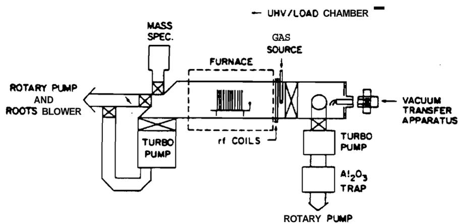
Figure 2.6 UHV/CVD system schematic [13].
