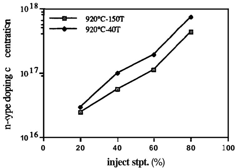
Figure 4.8 (b) Phosphorus concentration vs. dopant set point at 920°C as determined by four point probe measurements.
