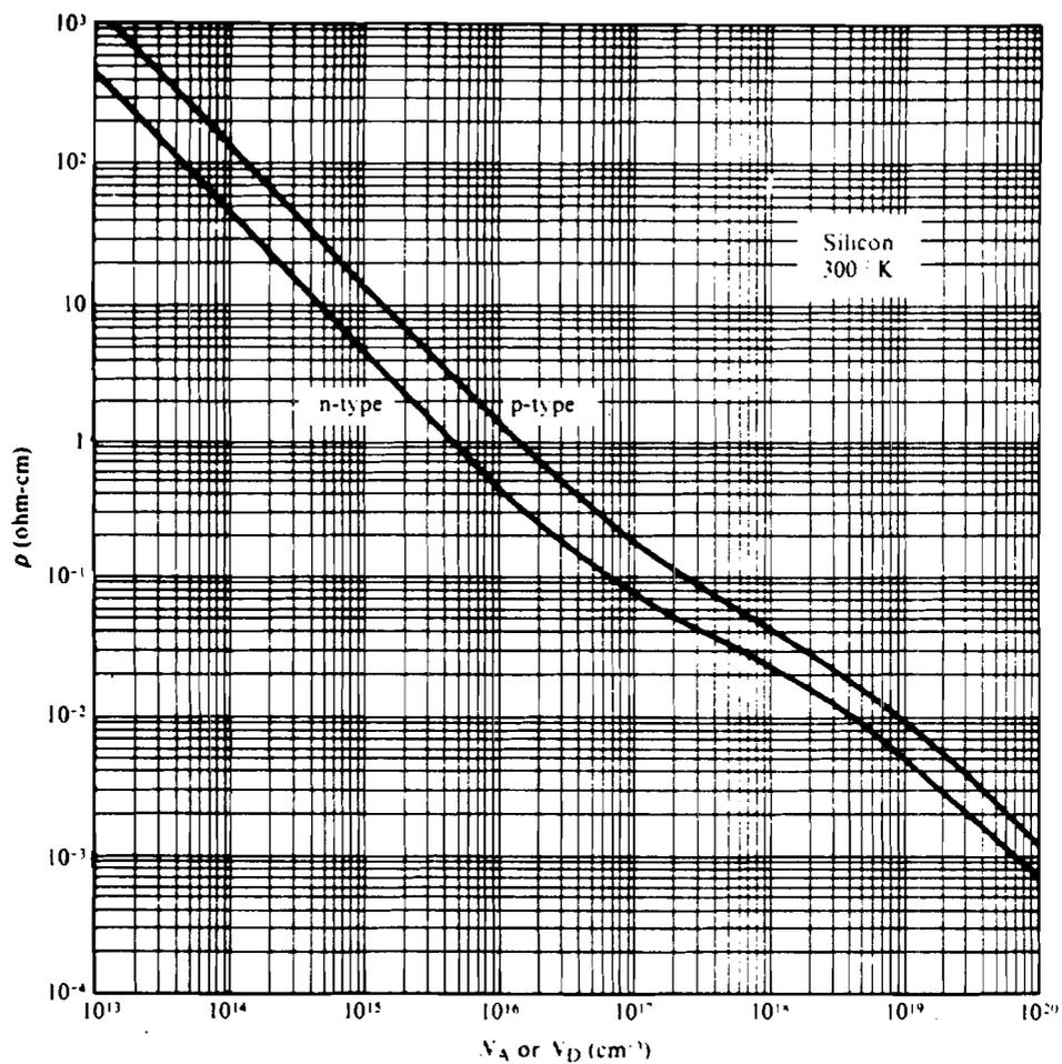
Figure 3.7 Resistivity versus doping concentration at room temperature for p-type (boron-doped) and n-type (phosphorus-doped) silicon [72].
