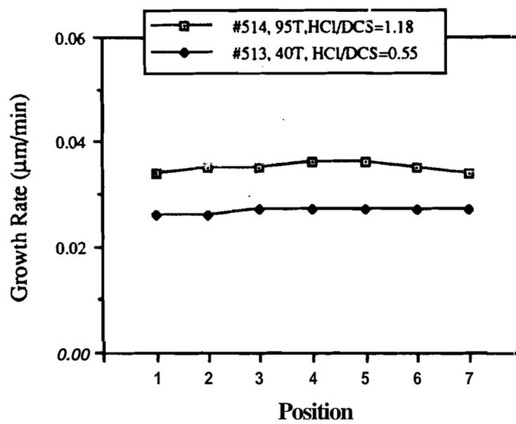
Figure 4.4 (c) Selective epitaxy growth rate profiles on oxide-patterned wafers at 870°C and various pressures.
