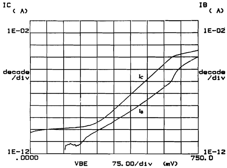
Figure 4.15 (a) Measured  $I_B$  and  $I_C$  versus  $V_{BE}$  characteristics for a representative bipolar transistor fabricated in 970°C-40T SEG.
