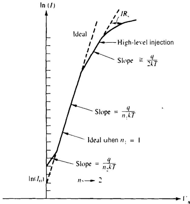
Figure 3.6 Forward-biased current-voltage characteristics of a diode [71].
