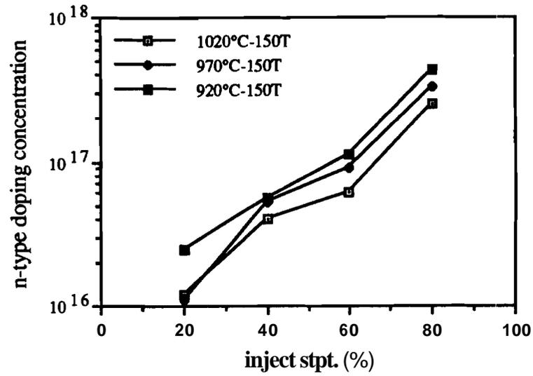
Figure 4.8 (c) Phosphorus concentration vs. dopant set point at 150 torr as determined by four point probe measurements.
