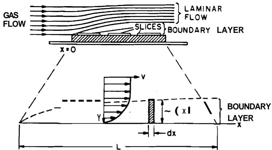
Figure 2.4 Development of a boundary layer in gas flow over a flat plate and expanded view of the boundary layer [18].
