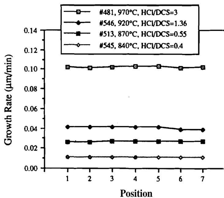
Figure 4.3 (c) Selective epitaxy growth rate profiles on oxide-patterned wafers at 40 Torr and various temperatures.
