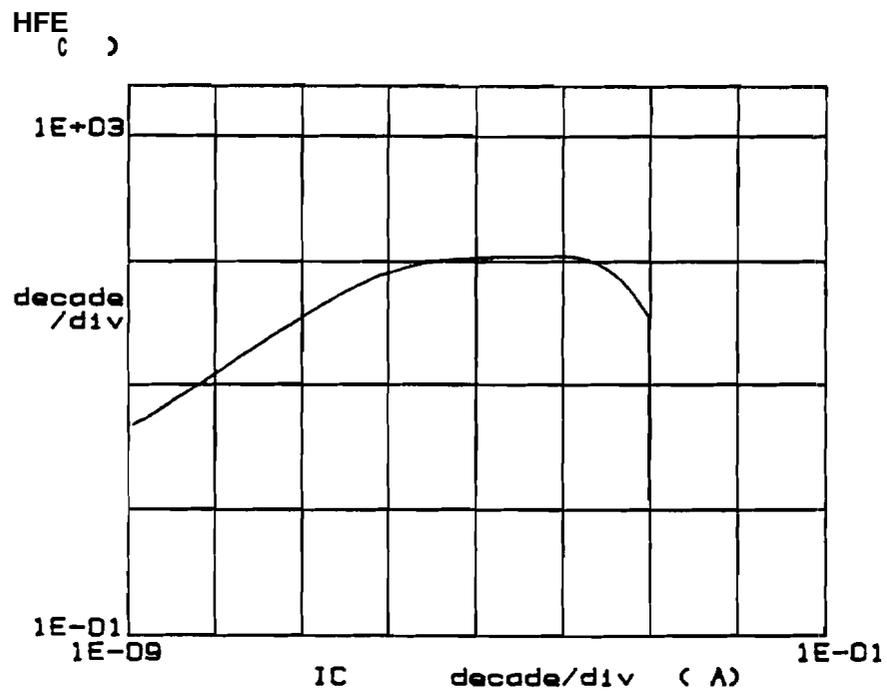
**Figure 4.16(b)** Measured current gain ( $\beta$ ) versus collector current ( $I_C$ ) characteristics for a representative bipolar transistor fabricated in silicon substrate.
