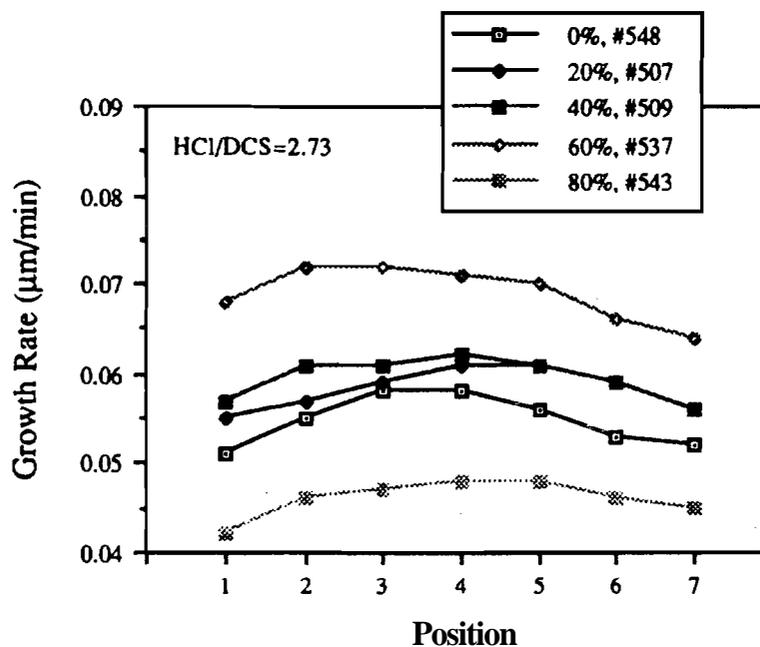
Figure 4.6 (d) Selective epitaxy growth rate profiles on oxide-patterned wafers at 920°C, 150T, and various PH<sub>3</sub> dopant set points.
