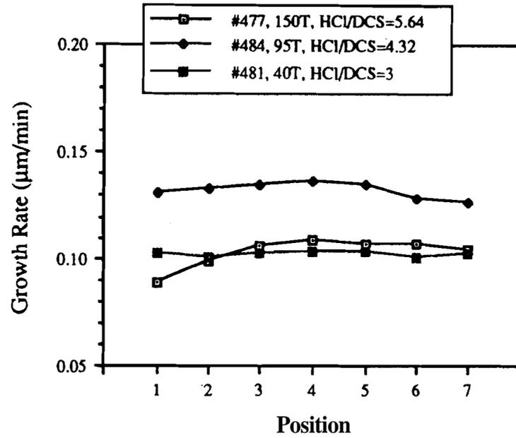
Figure 4.4 (a) Selective epitaxy growth rate profiles on oxide-patterned wafers at 970°C and various pressures.
