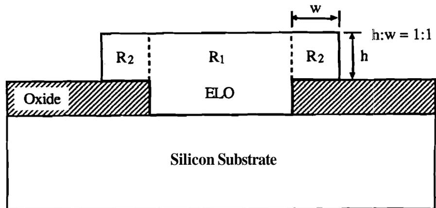
Figure 4.9 (b) A simple modification model of ELO for determining resistivity.
