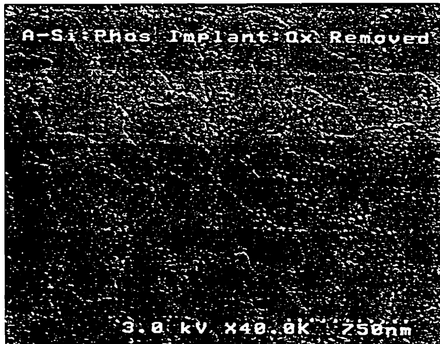
Fig. 3.3 Phosphorus implanted amorphous silicon after 250 Å oxidation was removed.
