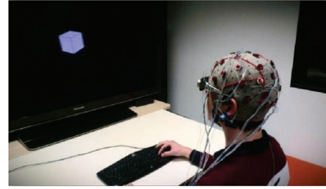
FIGURE 4: Setup of the experiment, with a subject being presented with stereoscopic images while his EEG signals are being recorded.
