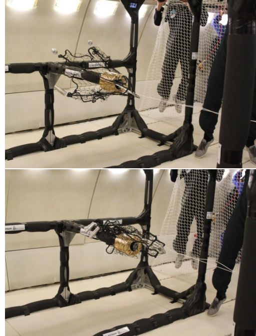
Fig. 18: Net Testing: Novespace A300 Parabolic Flight. Target capture and closure of 1 m net demonstrated in parabolic flight (capture top, closure bottom).
