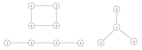
Figure 6: Examples of conflict graph: the square, the 4-link line and the 4-link star.
