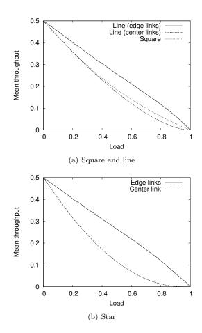
Figure 7: Mean throughput in 4-link networks.
