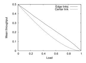
Figure 5: Mean throughput in the 3-link line.
