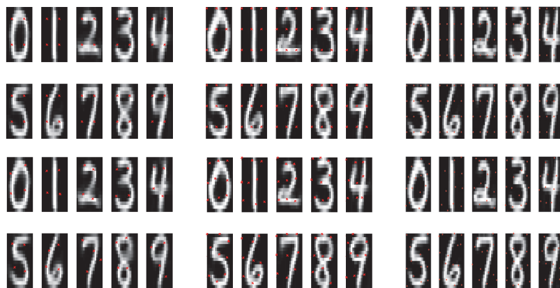
Figure 2. Estimated templates with varying numbers of control points: 4 (left), 9 (middle), and 16 (right) with either fixed (top) or estimated (bottom) control points positions.
