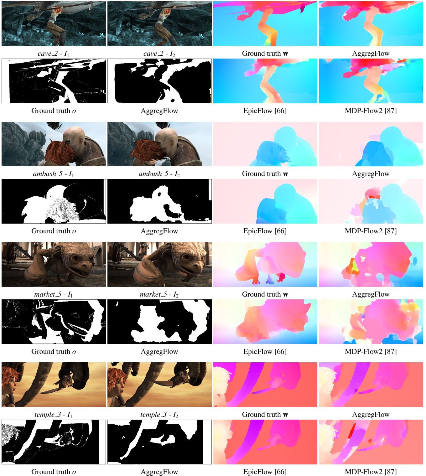
Figure 5: Comparative evaluation with EpicFlow [66] and MDP-Flow2 [87] on several sequences of the MPI Sintel dataset. Every first row from left to right: successive input images, ground truth motion field, motion field computed with AggregFlow. Every second row from left to right: ground truth occlusion, occlusion map computed with AggregFlow, motion fields computed respectively with EpicFlow [66] and MDP-Flow2 [87].
