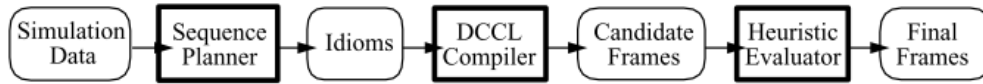
Figure 2.21: Pipeline of the CPS presented by [CAH*96]. After finding all candidate idioms from the simulation data using a sequence planner, the CPS compile them to generate all candidate frames. Finally, the candidate frames are evaluated to compute the best possible edit.
