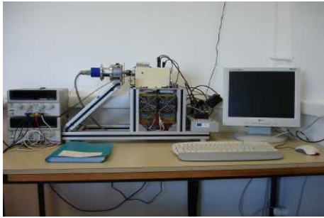
Fig. 3. Stepper-motor test bench.
