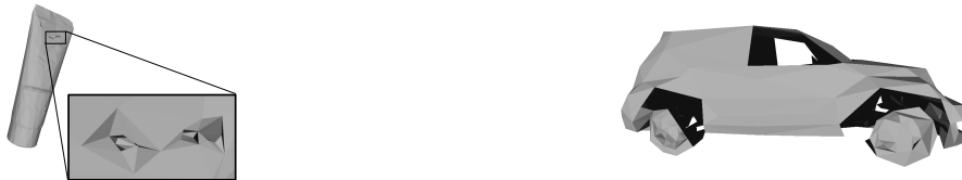
Figure 8: Left: KIT Toothpaste is a non-manifold mesh. Note that the zoomed-in section of the object is shown inside the rectangle. Right: KIT ToyCarYelloq has several holes.
