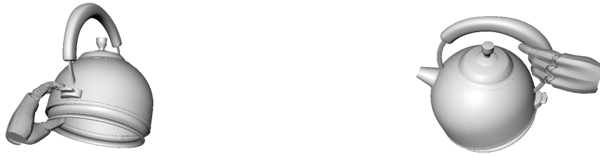
Figure 16: Left: A grasp synthesized by the generic grasp planner in Simox for a kettle. Right: A grasp synthesized by our cord-driven grasp planner that grasps the kettle handle.
