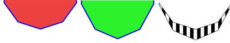
Figure 7: The two 2D polygons shown in the first two subfigures originate from the intersections shown in the right subfigure of Fig. 6. After performing the Boolean XOR operation on these polygons, the polygon clipper outputs one 2D polygon (the striped region shown in the third subfigure).
