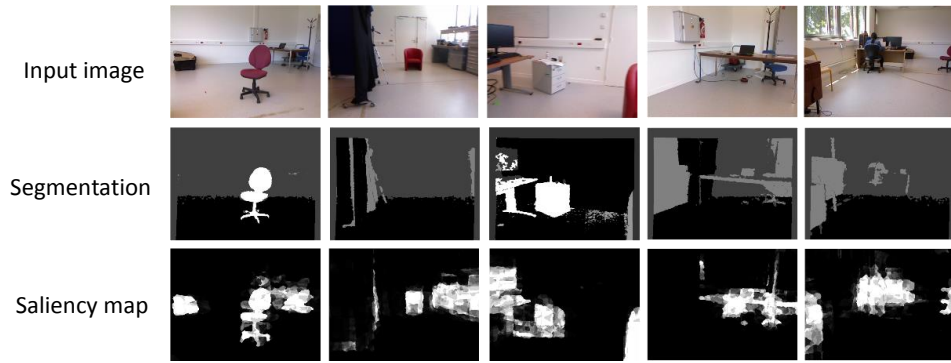
Fig. 2. Saliency and segmentation results for a few examples. First row: the RGB image. Second row: the segmentation result, obtained from the depth input only. Grey areas of the segmentation images are pixels labeled as unavailable (dark gray), or undetermined (light gray). Third row: the saliency result, obtained from RGB features only. The classifier outputs for each pixel a fuzzy score between 0 ( not salient ) and 1 ( salient ). Note that the classifier is able to generalize so as to retrieve the saliency of data that is unavailable in the depth input.
