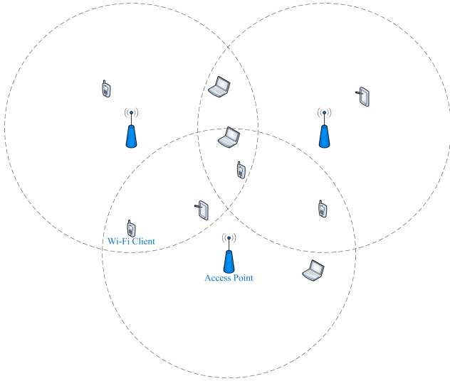
Fig. 2. Wi-Fi network having several clients
