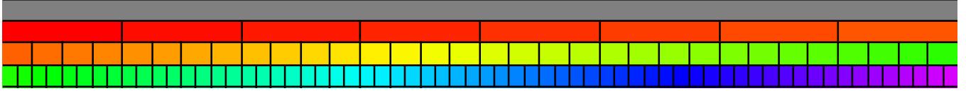
Fig. 4. Color code used to show our hierarchical segmentation results for a 3-deep tree where nodes in 0-th, first and second layer have respectively 8, 4 and 2 children each. Each node corresponds to a different color of the HSV colormap.
