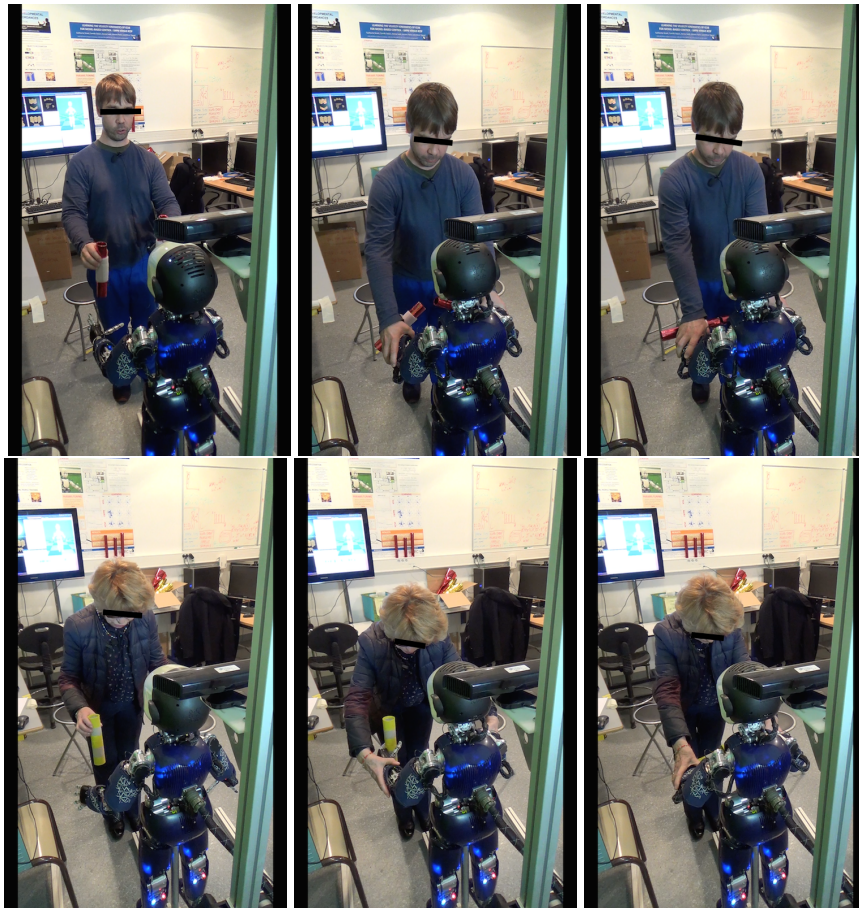
Fig. 7 Some participants performing the assembly task (screenshots from the front camera). The three images show the participants giving the cylinders to the robot (left), grabbing the robot arms (center) then moving the arms to align the cylinders (right).
