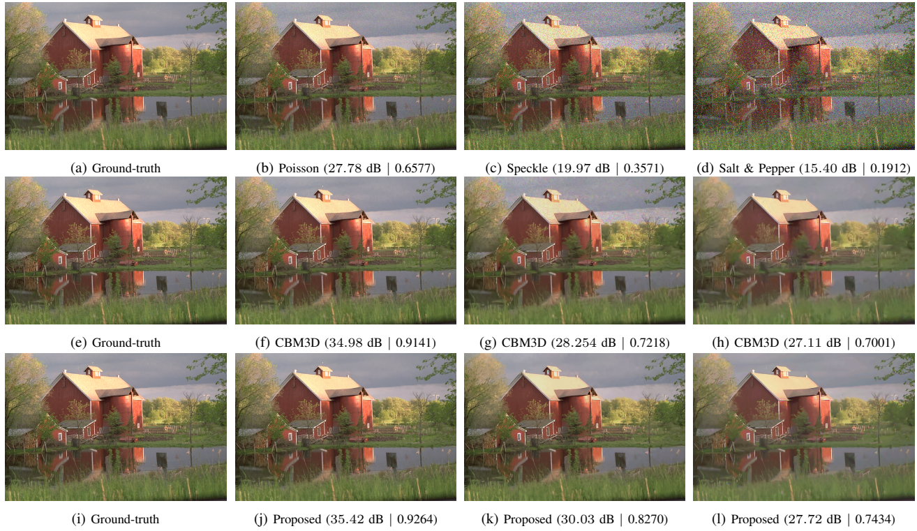
Fig. 7: Denoising results with different types of noise. The first line presents noisy results, the second and third lines represent respectively denoising results produced with CBM3D and the proposed method with PSNR and SSIM. As can be seen, the proposed approach produces high-quality restoration results.
