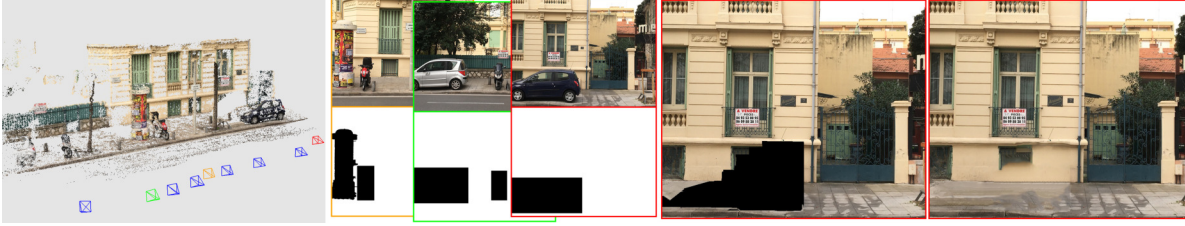
Figure 1. (a) 3D reconstruction from multi-view input image dataset (b) Input images above, input masks below (c) Result of reprojection and mincut, remaining black pixels will be filled through patch-based inpainting (d) Inpainted result.
