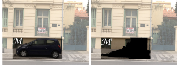
Figure 2. Left: A crop of an input image showing the mask \mathcal{M} as a dark region. Right: The resulting image \mathcal{I}_r from reprojection into \mathcal{M} . The non-black pixels within the box are the region \mathcal{M}^r .
