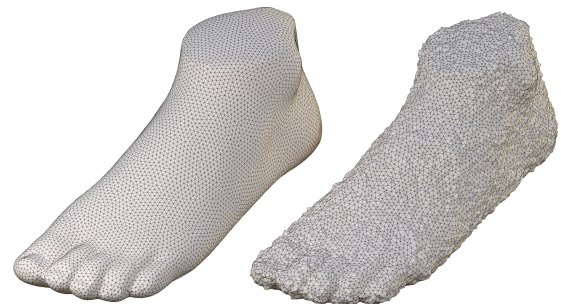
Figure 6: Connectivity shape illustrated with the foot model. The original immersion (left) has its vertex positions entirely removed. Using only the combinatorics, we can approximate them (right).
