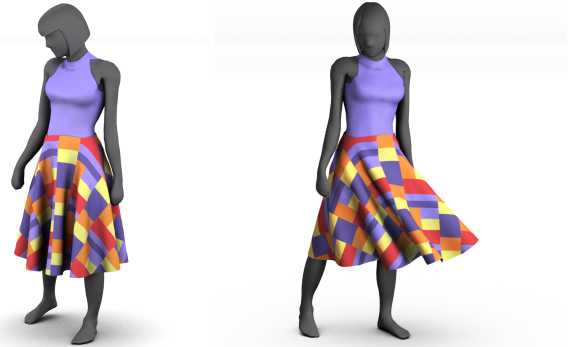
Figure 1: Breathing physics into a purely geometric garment directly modeled in 3D under gravity. From the 3D mesh of the cloth and the body mesh, our method automatically infers the rest pose of a cloth simulator such that a stable equilibrium of the cloth simulator under gravity and frictional contact closely matches the input geometry. Starting from this input pose, the cloth can then be animated in a plausible manner; for instance under wind.
