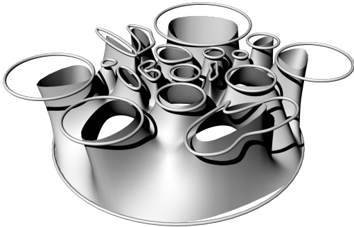
Figure 10: Rendered view of the initial T-spline surface along with the input contour-set.
