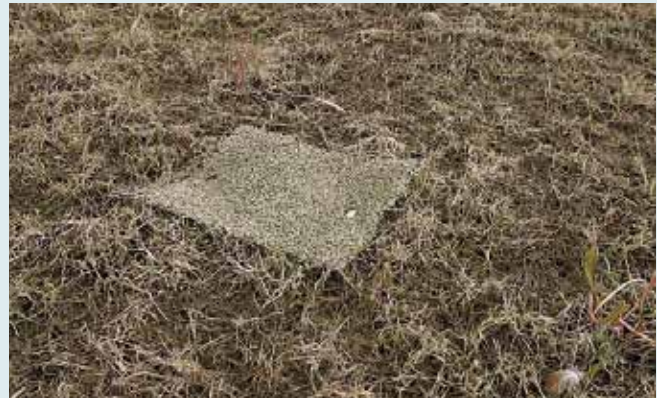
Small pieces of astro turf (weighed in advance and pinned down with pegs), called ‘sedimats’ are used to capture sediment deposited during a flood. They must be placed on site before a flood and then collected and removed to a lab afterwards. © Mike Dodd
