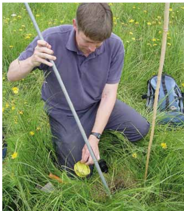
Monitoring soil: measuring water levels in a dipwell using a buzzing stick. © Emma Rothero
