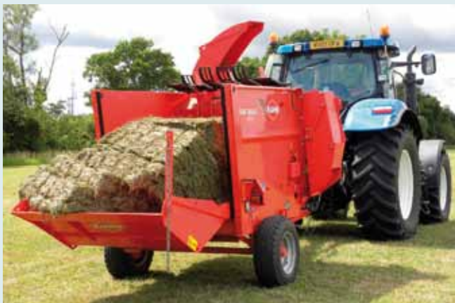
The bale is loaded into the rear of the spreader, chopped and then spread over the grassland through a funnel. The angle of the funnel and flow rate are adjustable, allowing the depth of the green-hay layer and the area of distribution to be altered. This method is quick and efficient. © Catherine Hosie
