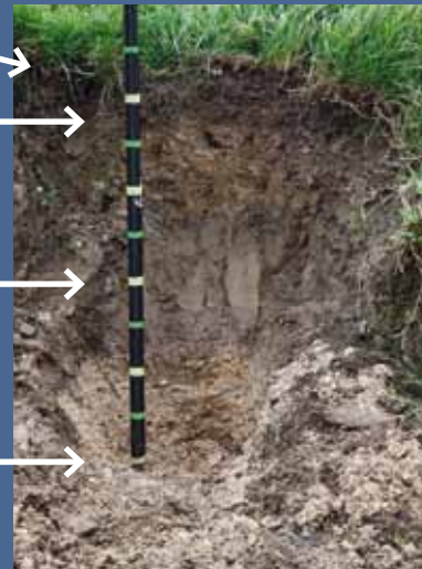
Soil profile through the bank of the River Churn (adjacent to North Meadow). River banks often provide the opportunity to see the thickness of the various layers and confirm the presence of terrace deposits. © Mike Dodd
