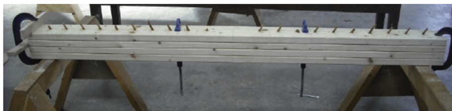
Fig. 7. Dowel laminated timber beam fabricated by O'Loinsigh et al. (2012a).
