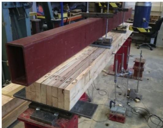
Fig. 4. Four-point bending test setup on a dowel laminated timber beam by Plowas et al. (2015).
