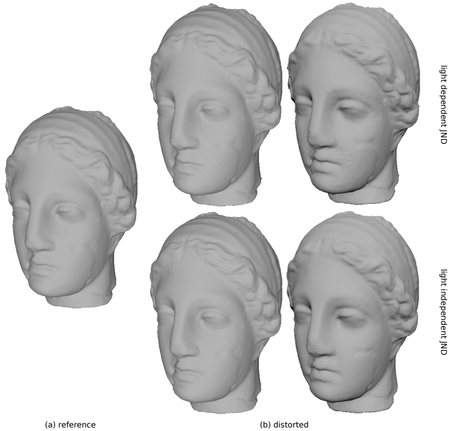
Figure 9: A vertex noise at the JND level computed in a light dependent mode might become visible when the light direction is altered. This is not the case for JND computed under light independent mode.
