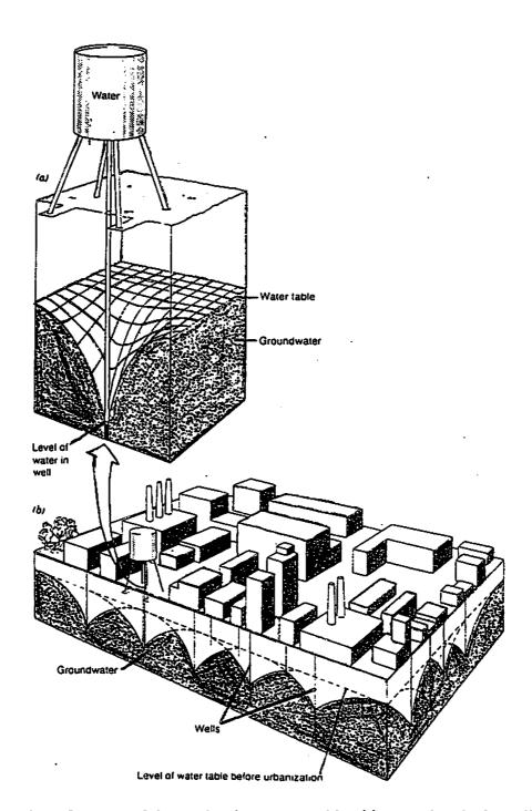
Figure 3.10. Formation of a cone of depression in a water table: (a) around a single well; (b) intersecting cones of depression resulting from many closely spaced wells in an uranized area. Source: Marsh, William M., *Earthscape: A Physical Geography*, 1987. (#21)
