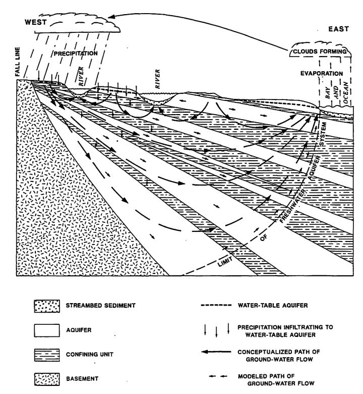
Figure 3-5. Generalized hydrologic cycle for York-James Peninsula. Source: U.S. Geological Survey WRI Report 88-4059, 1988. (#39)
