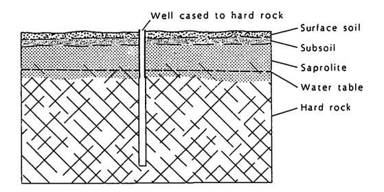
Figure 3.9. Typical subsurface cross section showing the character of materials penetrated by a well in crystalline terrane. (LeGrand, 1960.) Source: U.S. Geological Survey WRI Report 85-4235, 1985. (#38)
