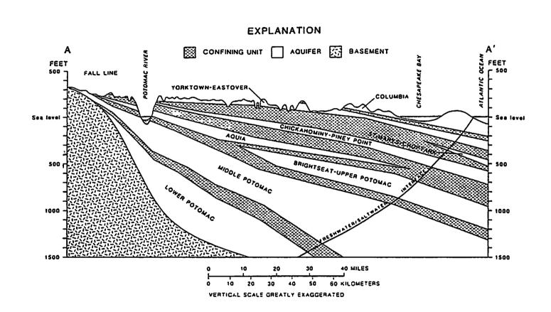
Figure 3.6. Hydrogeological Section: Coastal Plain Province. Source: U.S. Geological Survey WRI Report, 87-4049, 1988. (#40)
