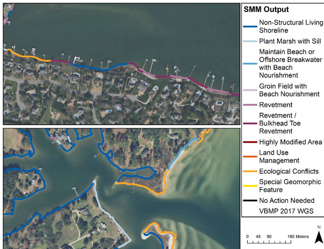
Fig. 4. Sections of the shoreline of City of Virginia Beach (top) and Gloucester County (bottom), Virginia, displaying the SMM outputs. Background image: VBMP2017/VBMP2017_WGS—Virginia Geographic Information Network (VGIN).
