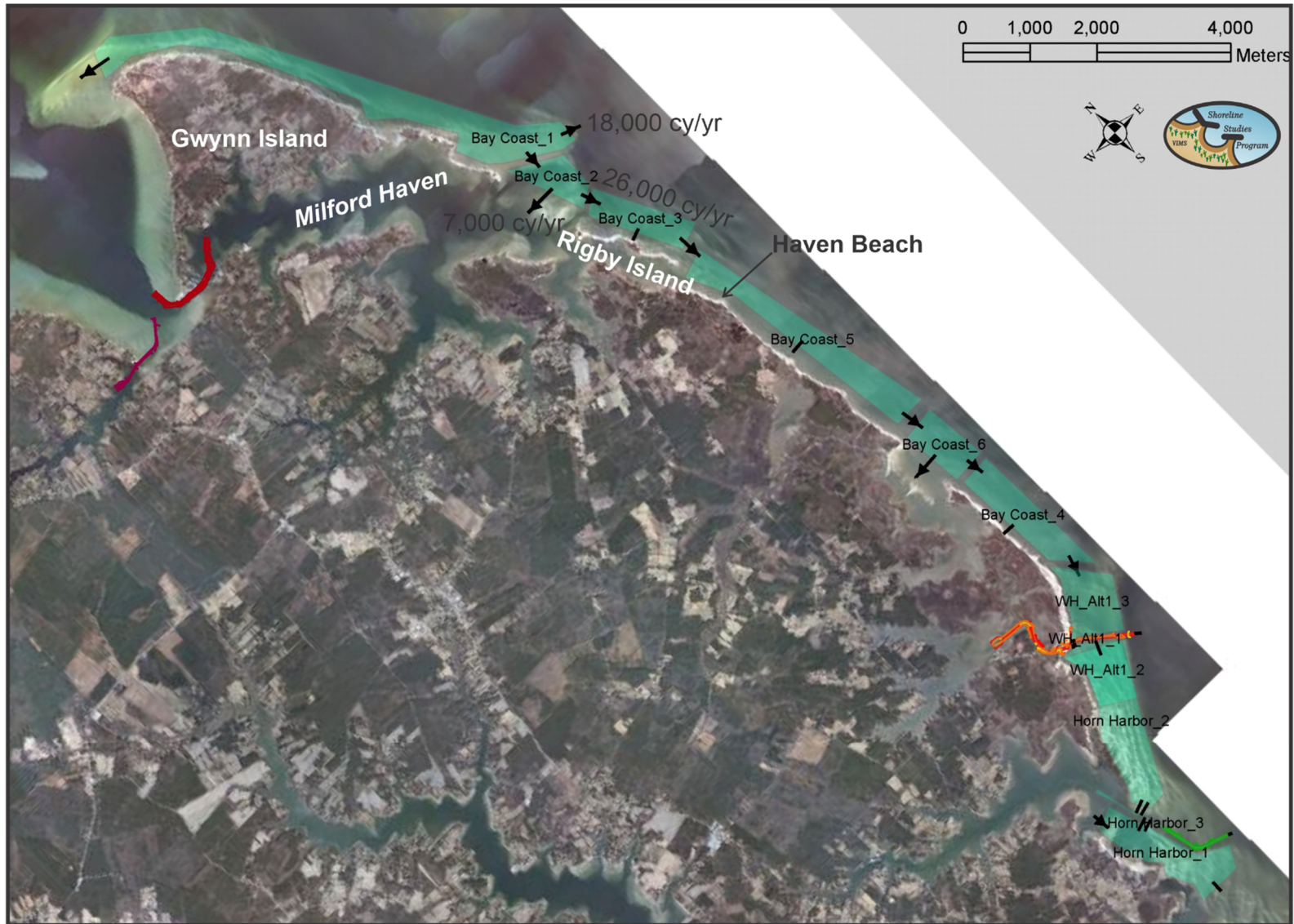
Figure 29. Unpublished sediment budget for the Mathews County Bay coast. VIMS, Shoreline Studies Program.
