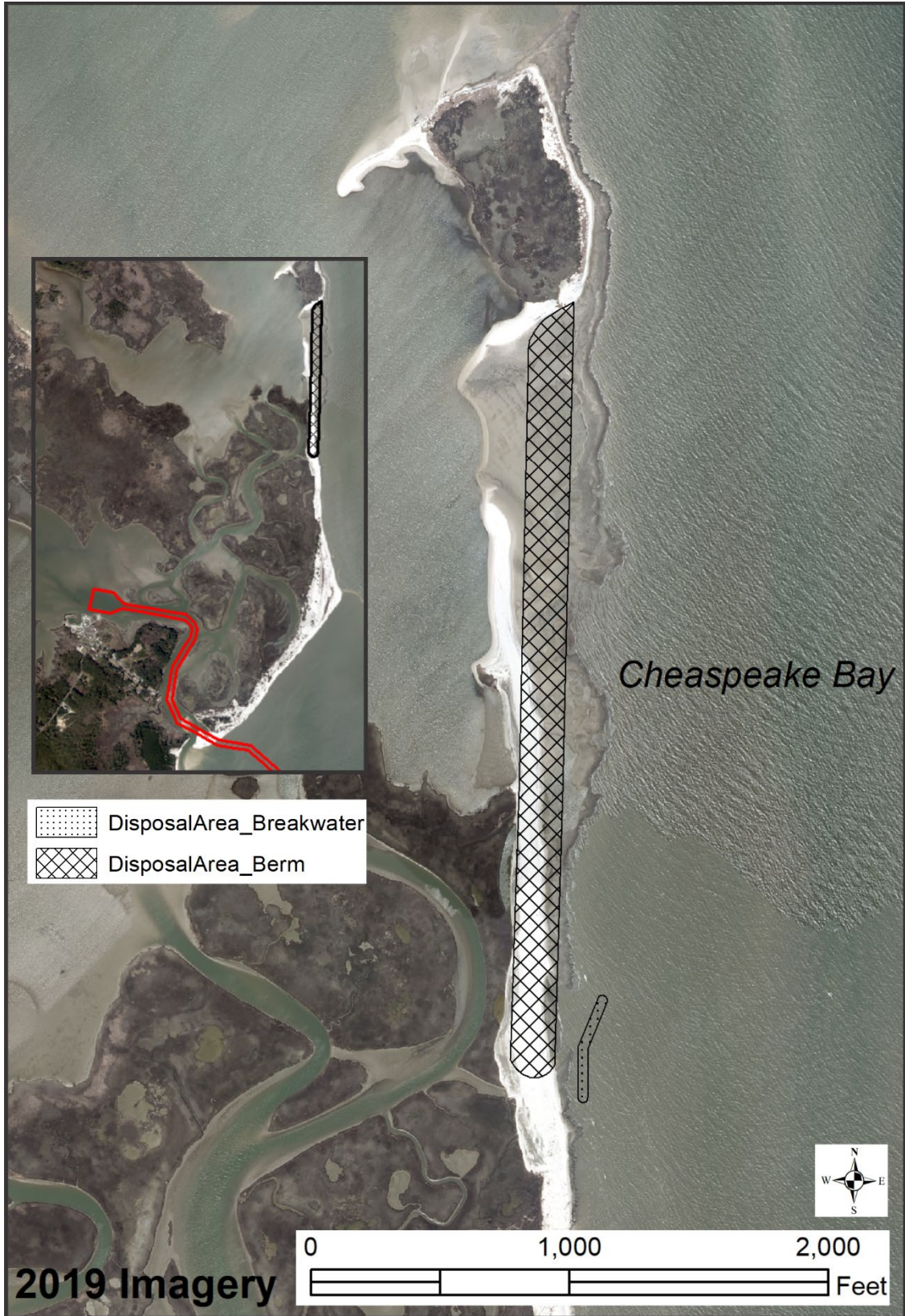
Figure 22. Proposed placement for sandy material beneficial use and proposed nearshore breakwater. The inset shows location relative to the channel. Pumping distance is about 1.5 miles.
