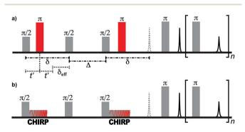
Fig. 1 (a) Traditional relaxation-compensated  $D-T_2$  pulse sequence. (b) Ultrafast  $D-T_2$  pulse sequence. In the single-sided instrument, a constant field gradient is present throughout the experiment.
