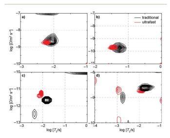
**Fig. 3** Traditional (black) and ultrafast (red)  $D-T_2$  correlation maps of (a) water doped with copper(II) sulfate, (b) ethylene glycol, (c) glycerol, and (d) water in 4 Å molecular sieves. Values for *D* and  $T_2$  for these samples are given in Table S3.<sup>†</sup>
