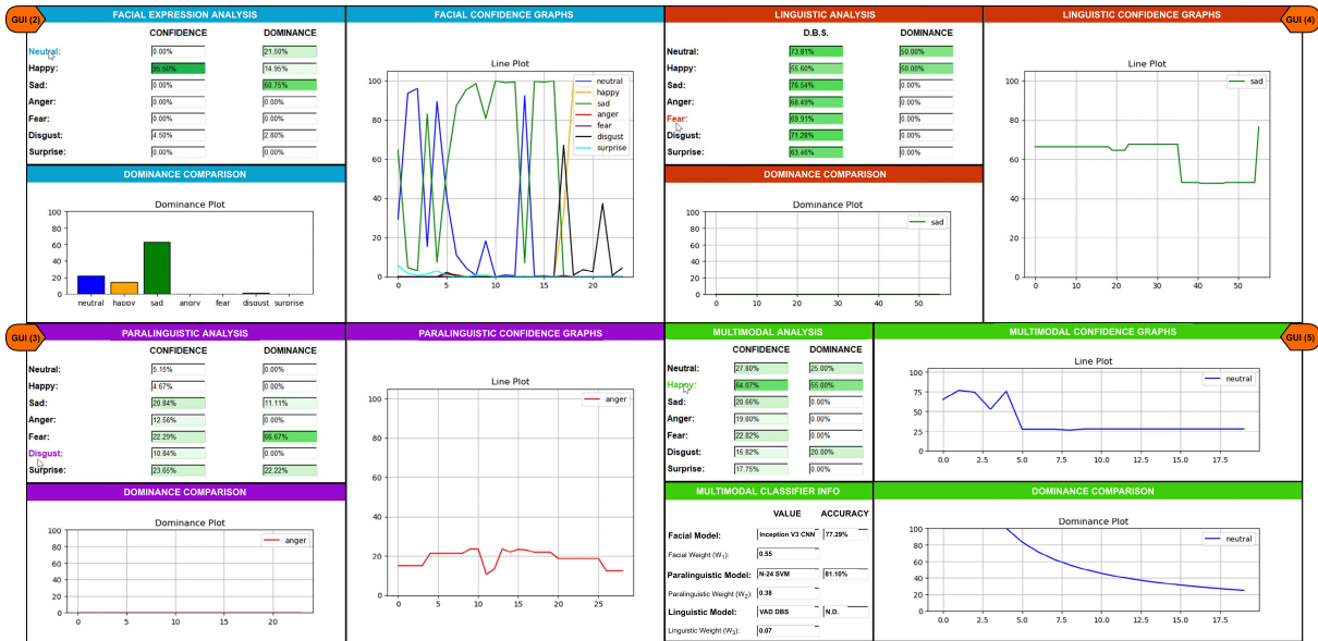
FIGURE 15. Overview of the multimodal ASA monitoring windows embedded in the ASAM. These windows are accessible through their corresponding “Analyse Data” buttons as shown in Fig. 14. The Multimodal Analysis window – GUI (5) is opened in parallel to the GUI (1) window shown in Fig. 14. Tetradic colour theory was chosen for GUI window design where: CYAN = Facial Expression Analysis, ORANGE = Linguistic Analysis, PURPLE = Paralinguistic Analysis and LIME.
