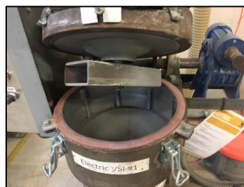
Figure 3-6. VSI crusher located at Gekko Pty Ltd
