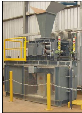
Figure 3-5. Polysius SMALLWAL HPGR unit located at SGS Australia Pty Ltd
