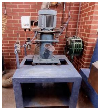
Figure 3-3. Laboratory Sala mortar cone crusher located at CSIRO
