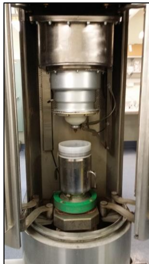
Figure 3-7. SELFRAG process vessel in association with the electrode located at the JdLC
