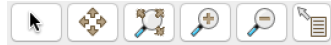
Figure 5.4: Buttons related to the map content navigation and selection on the map panel in the order of road edge selection, map scrolling, fitting map to panel size, zoom in, zoom out and road asset information.
