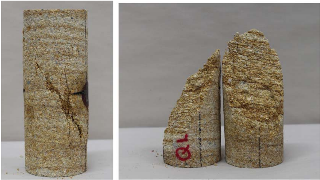
Figure 3.4 Example of moderately strong sandstone sample after uniaxial compressive strength test.
