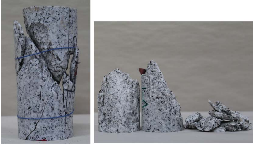
Figure 3.6 Example of granite sample after uniaxial compressive strength test.
