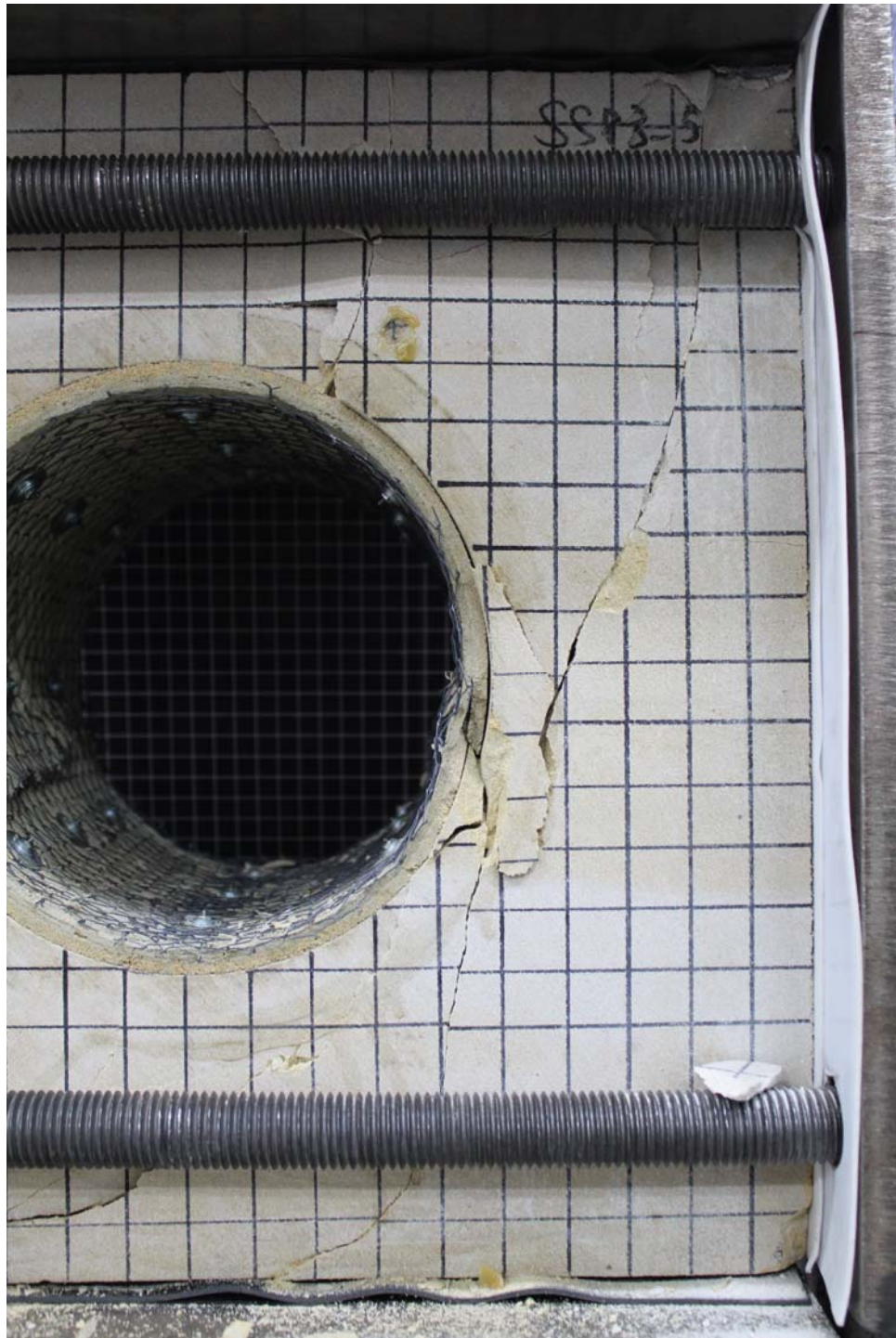
Figure 8.41 The shear failure on the pillar (Specimen No.14).
