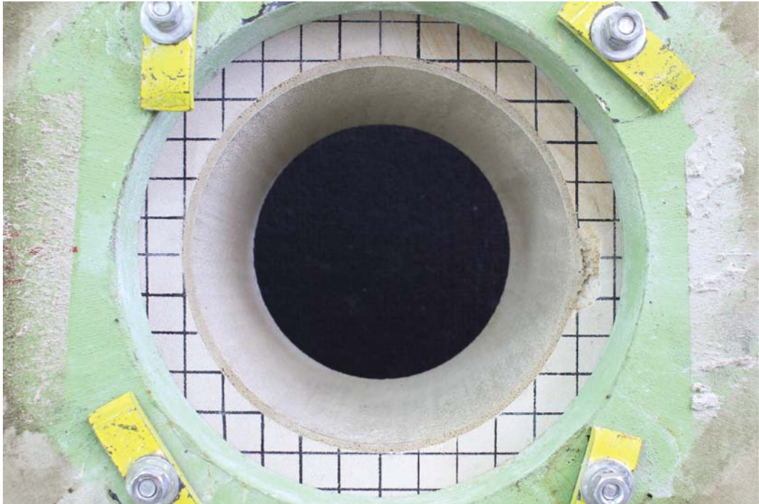
Figure 4.22 A scaled down tunnel with a 5 mm thickness shotcrete layer after curing.
