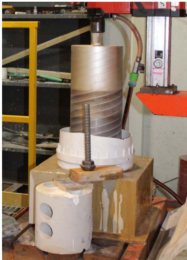
Figure 4.2 Example of 200 mm core drilling into a sandstone block.
