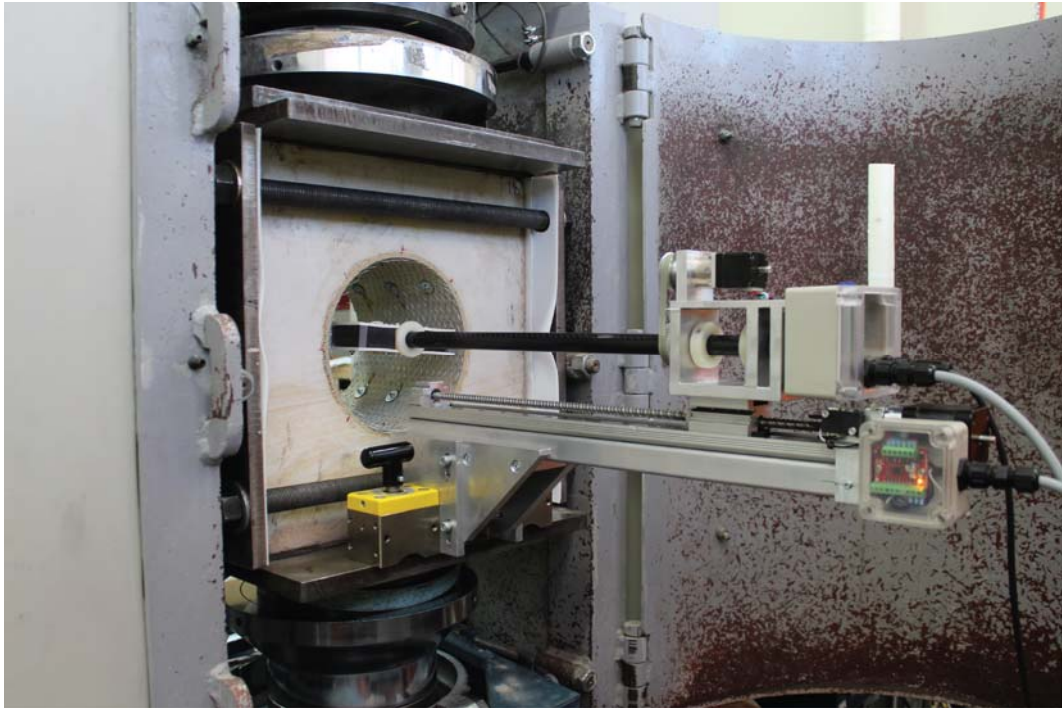
Figure 5.10 An example of the laser scanner setting within a specimen sample.
