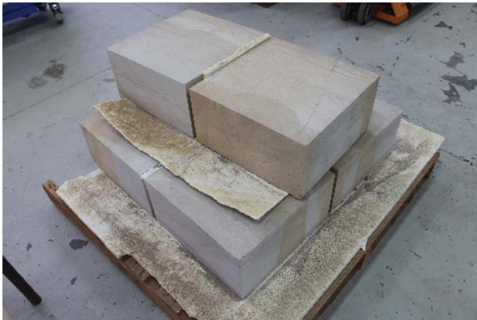
Figure 4.1 Sandstone block (strong) before the drilling process.
