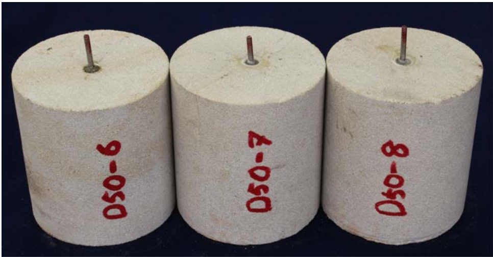
Figure 4.10 The sample specimen with the rock bolt prior to the tensile test.
