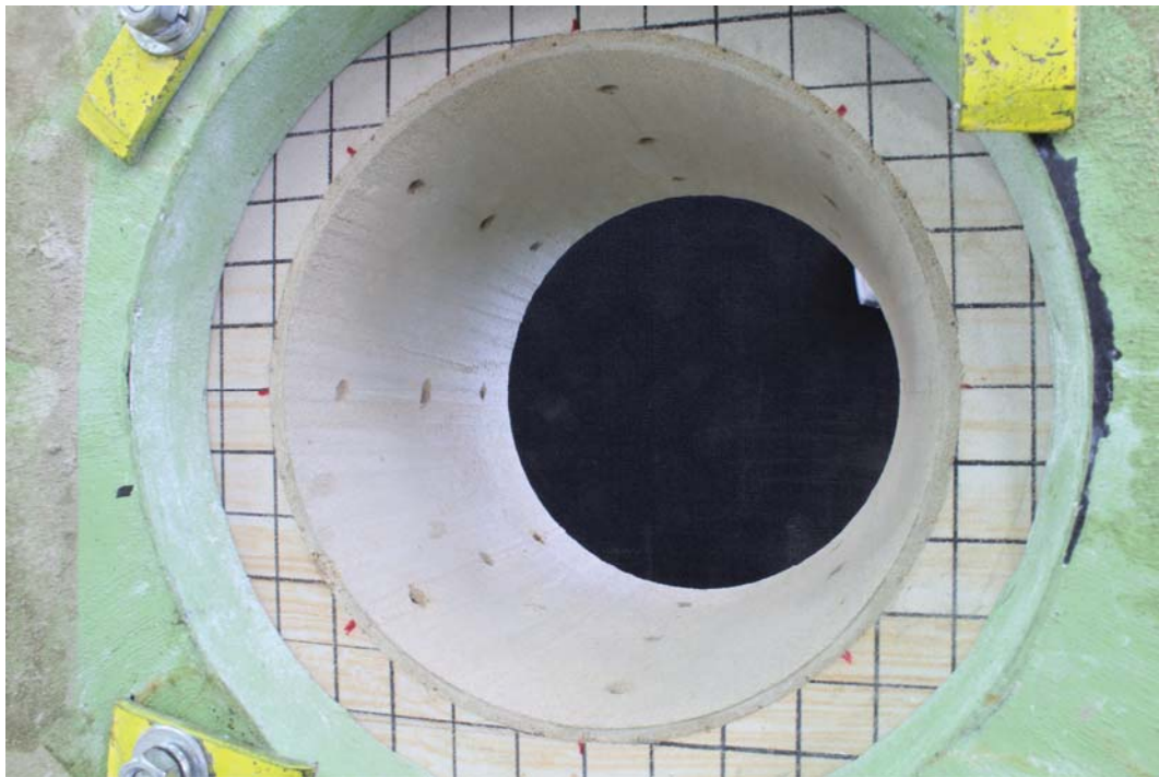
Figure 4.23 Re-drilled boreholes after shotcrete application.
