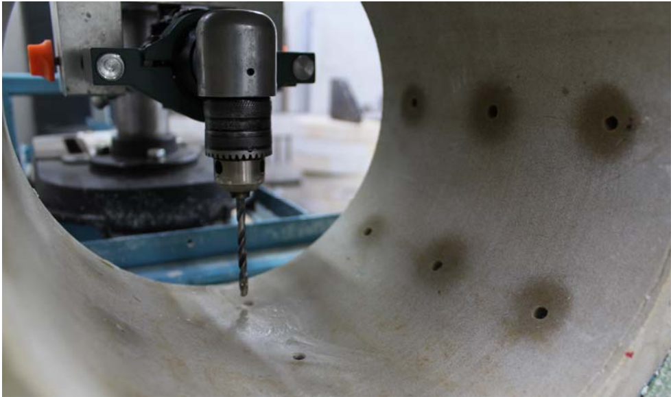
Figure 4.6 Borehole drilling process using a 5mm diamond drill bit.
