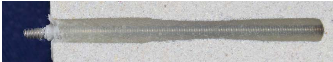
Figure 4.12 Long view of broken threaded steel bar after tensile testing.
