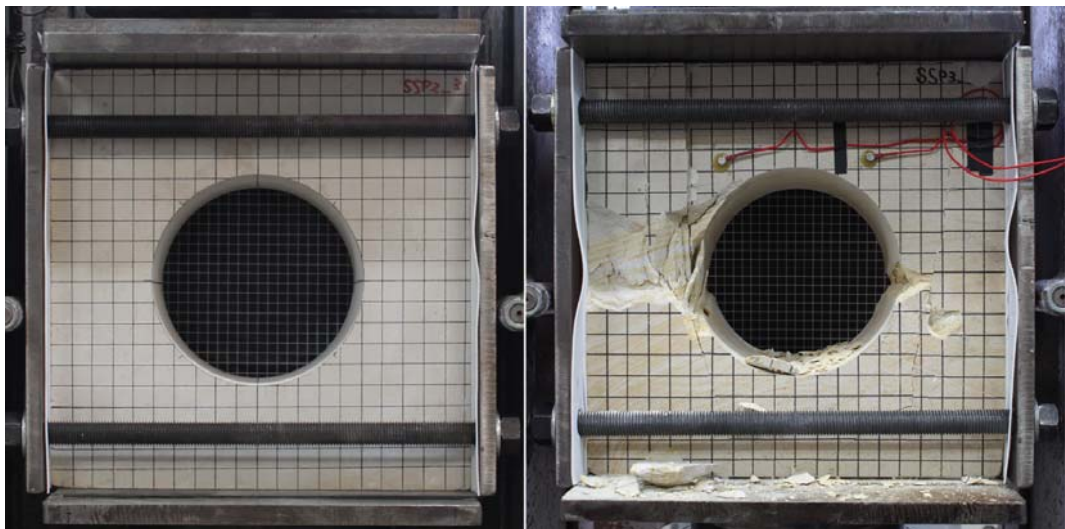
Figure 6.2 Typical unsupported tunnel and pillar geometry tested (grid size 20 mm x 20 mm), before and after failure.
