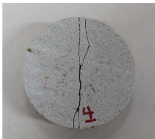
Figure 3.9 Example of strong sandstone sample after Brazilian test.
