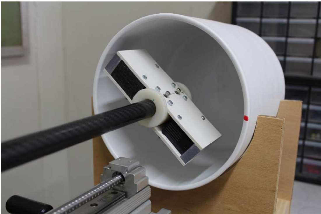
Figure 5.12 Reference scan testing using a ceramic tube.
