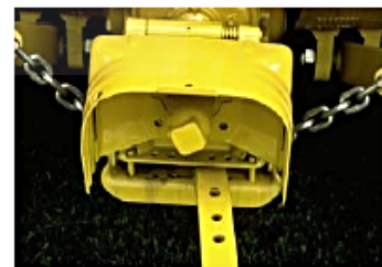
Figure 5.4.h. This PTO stub shaft is protected with a tractor master shield and stub shaft cover. To remove the stub shaft cover, grip the cover firmly and turn counterclockwise. Store the stub shaft cover where it will be available to replace when the job is done.
