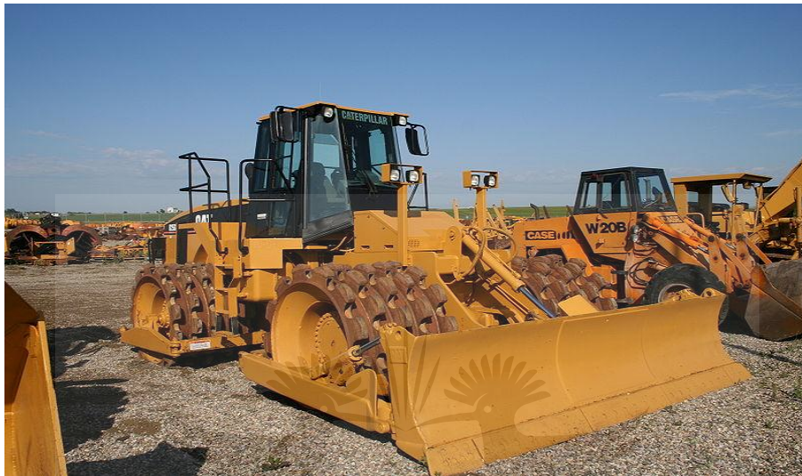
Figure 12: Tamping Foot Compactor.
