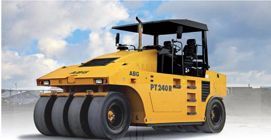
Figure 10: Pneumatic Tyre Compactors.
