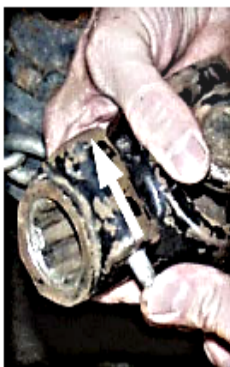
Figure 5.4.e. The push pin detent lock on the PTO driveline has a metal rod which fits in the PTO stub shaft groove to secure it. A firm grip is needed to press the pin. Do you have enough hand strength to push this pin in all the way?
