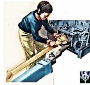
Figure 5.4.c. NAGCAT recommends that youthful farm workers wear snug-fitting clothes, non-skid shoes, and hearing protection while working around machinery. The youth's ability to lift and connect the PTO shaft must be evaluated by an adult who understands the physical development of children.
