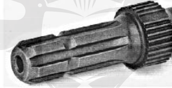
Figure 5.4.a. The 540 rpm PTO stub shaft has 6 splines or teeth and is 1 3/8 inch in diameter. Farm and Ranch Safety Management, John Deere Publishing, 1994. Illustrations reproduced by permission. All rights reserved.
