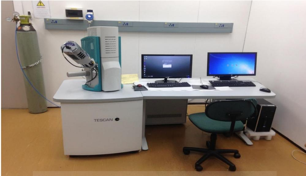
**Figure 3.8: TESCAN VEGA3 scanning electron microscope**
