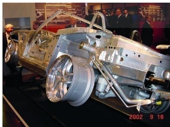
**Figure 2.4: A car featuring countless application areas of aluminium [23]**
