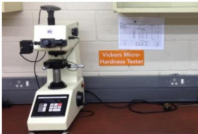
**Figure 3.9: TH713 Vickers microhardness tester**
