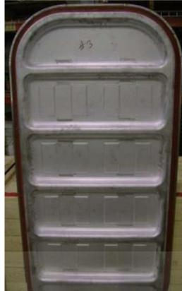
**Figure 2.12: Ship door manufactured from superplastic forming [29]**
