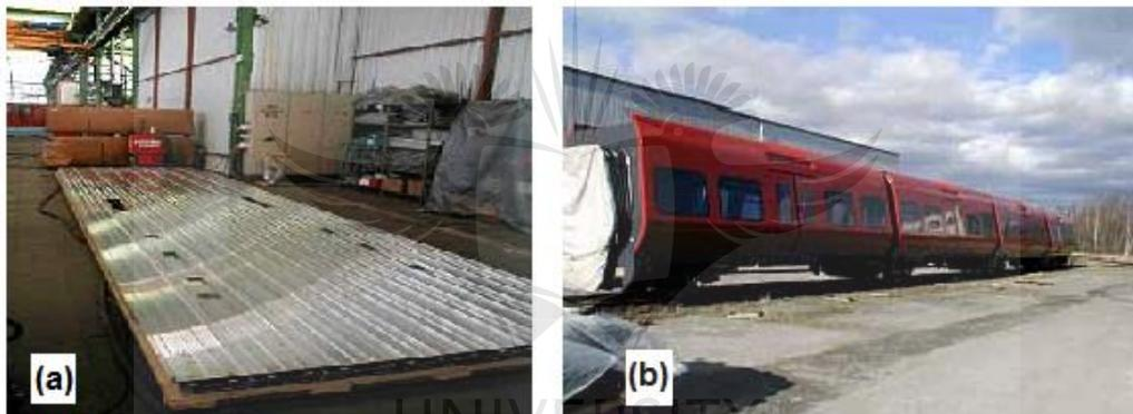
**Figure 2.10: Prefabricated FSW panels used for suburban trains [28]**
