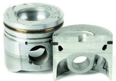
**Figure 2.11: Piston cast structure improvement with FSP [23]**
