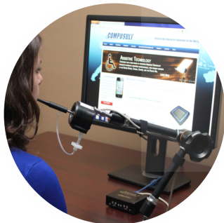
Figure 2.7. The Jouse 3, a sensitive joystick that is controlled through the mouth (Compusult, 2014)
