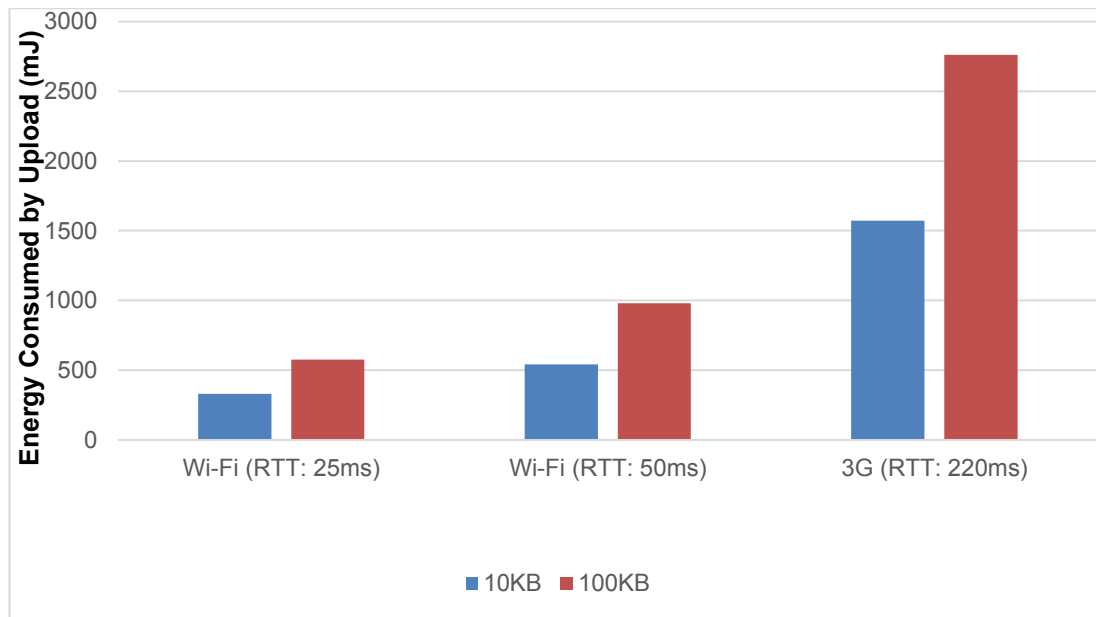
Figure 6.1 Energy Consumption: Wi-Fi vs. 3G
