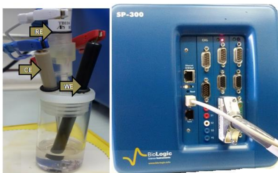
Figure 3.1 Structure of a three electrode operation electrochemical cell arrangement. The experimental cell consists a glass vial including a detachable lid having an inlet place as the electrode and gas cleaning. Here, the enough carrying electrolytes (to be contained) were chosen inside a glass vial and the reference electrode (RE), working electrode (WE) and counter electrode (CE) were dipped inside the cell.
