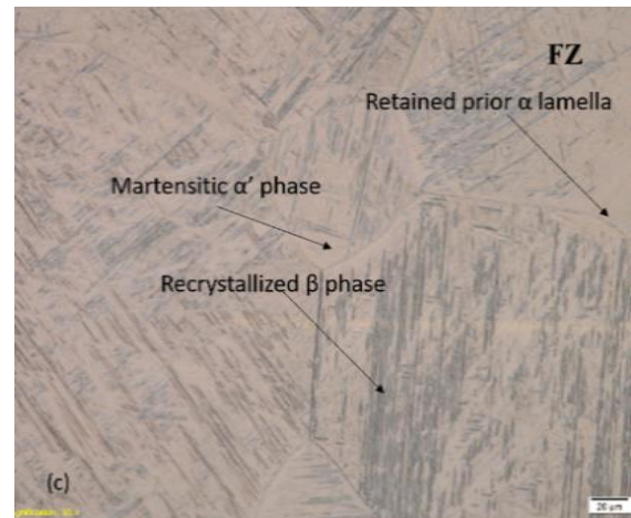
Figure 4. Optical micrograph of unpulsed TIG welding source [72]
