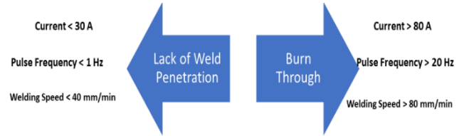
Figure 5. Cause and effect diagram of TIG welding parameters
