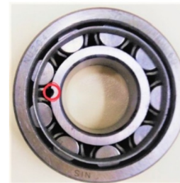
Fig. 2. Bearing with the inner race fault of 1 mm.
