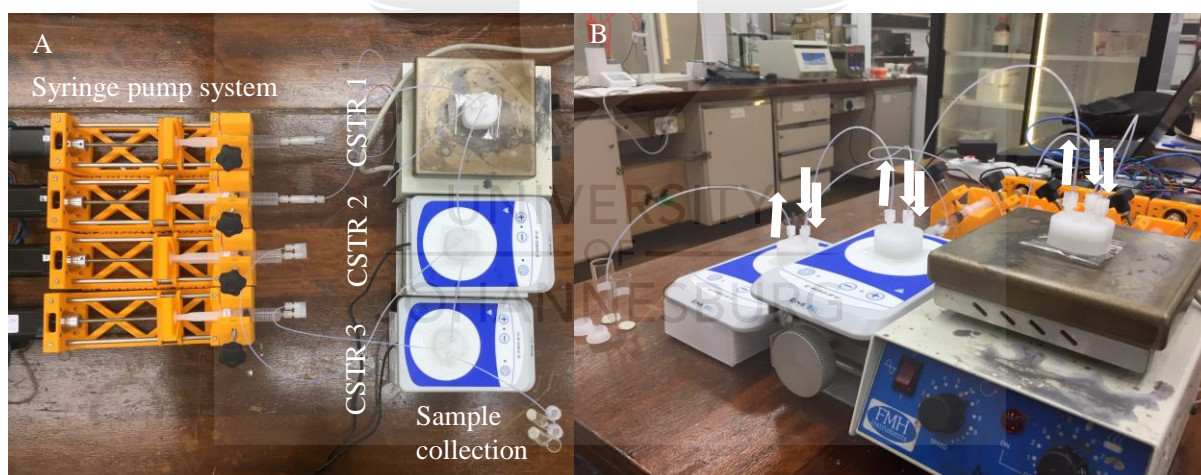
Figure 4.6: Set-up of the semi-automated 3D-printed flow system of the transesterification of edible oils. (A) A complete view of the flow system from above, consisting of the Poseidon syringe pump system, three CSTRs placed in series, and a sample collection zone. (B) A side view of the flow system where the arrows indicate the flow direction of the reagents and subsequent products. The downward pointing arrows shows the movement of fluid into the CSTRs originating from either the syringe pumps or the previous CSTR. The upward pointing arrows represent the movement of fluid exiting the CSTRs.
