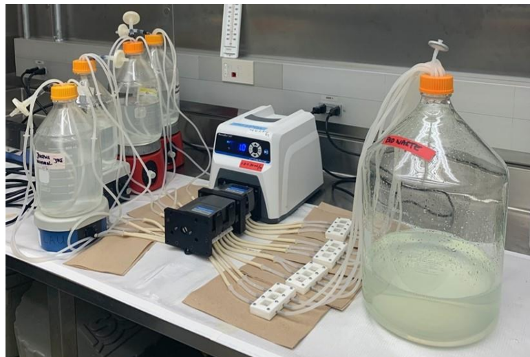
Figure 4.2: Experimental setup to cultivate biofilms with continuous flow in custom designed flow cells.
