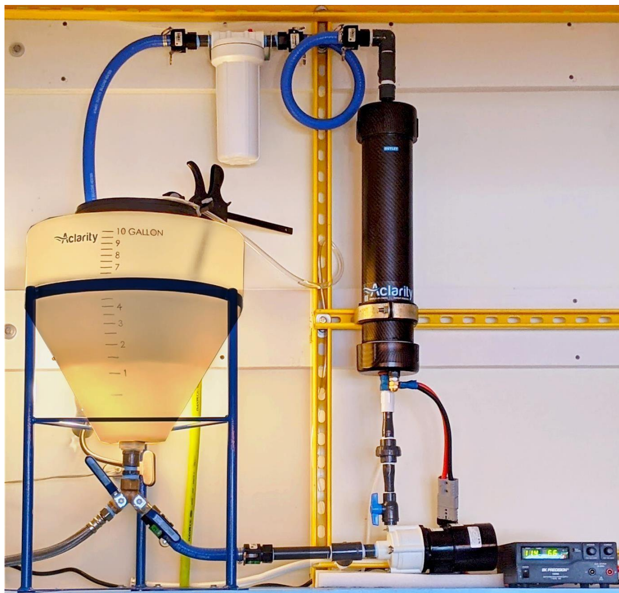
Figure 1: Experimental setup in the Aclarity laboratory with 10-gallon tank, pump, power supply, and electrochemical reactor
