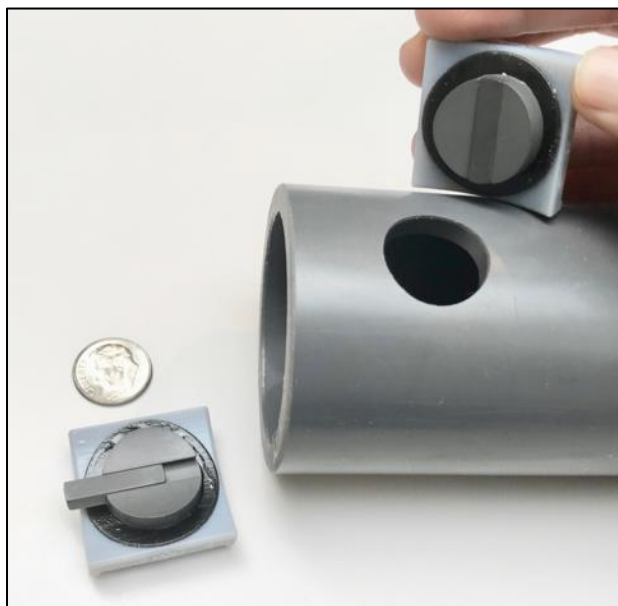
Figure 3. Biofilm sampler on left with an insert partially removed, with dime positioned above for scale. Biofilm samplers fit into holes drilled into pipe walls as demonstrated on the right. This design is based on the biofilm sampling coupon from the Pennine Water Group at the University of Sheffield (Deines et al. 2010).
