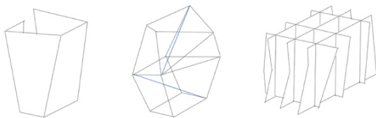
Fig. 4 Three structural types: strong skin, tectonic frame, and planar.
