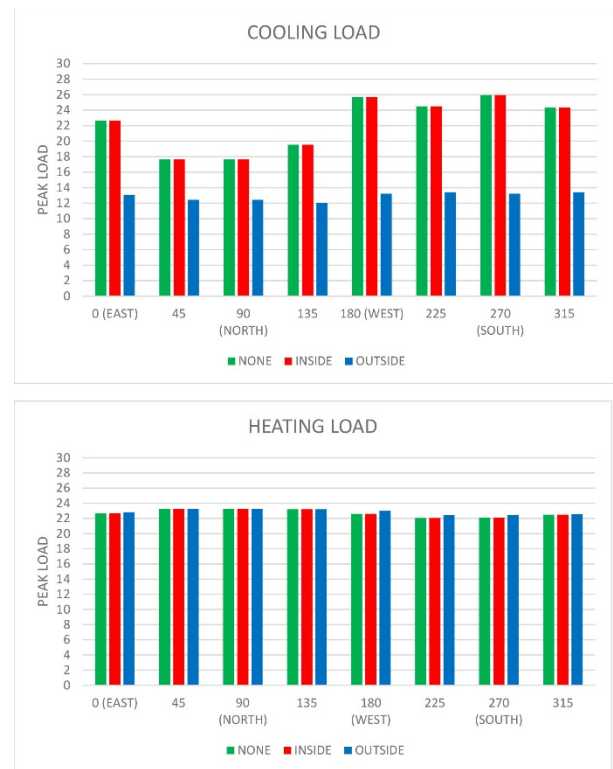
Fig 4. The peak heating and cooling load results from eQUEST. Cooling Load : While the inside and no louver options had similar results, the outside option reduced the peak cooling load for each orientation tested by half. Heating load : All three options performed similarly. Having louvers did not impact the heating load.
