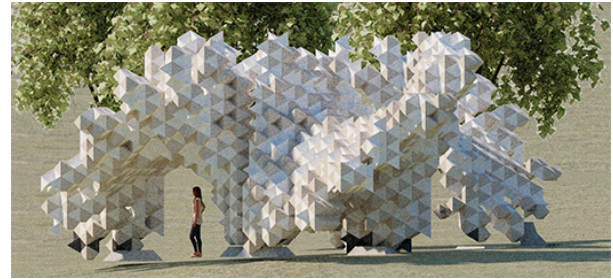
Figure 5. Equilateral four-sided pyramid packing structure of degradable (brown) and structural (white) composite blocks.
