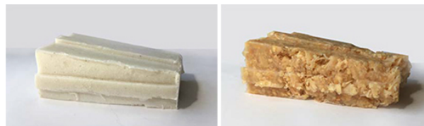
Figure 3. Compressive blocks of eggshell and agar agar (left) and sawdust and agar agar (right) in preliminary wedge-shape form with interlocking key.
