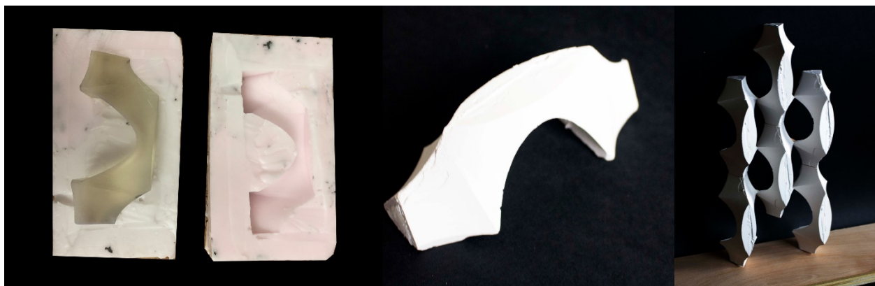
Fig. 6. (left) 3D printed reference piece placed in the two-part rubber mold; (middle) one cast plaster module; (right) assembly of cast modules. Work by (Image © Logan Osborn).
