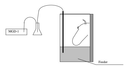
Figure 3. Measuring system when measuring cow's expiration air.
