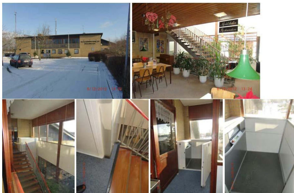
Figure 8. Overview of the architectural space: a modernistic floor layout allows automatically for level-free access and for vertical adjustments like low-rise elevators at the Knabstruphallen, Knabstrup, Denmark, (Photographs © author).
