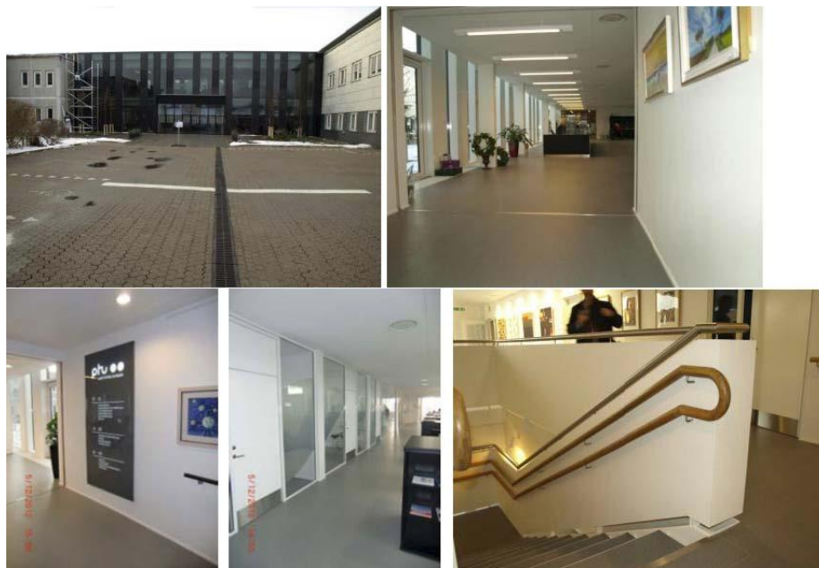
Figure 4. Overview of architectural space: level-free access from the outside to the inside, distinct signage in grey and white, glazing with opaque and transparent fields, and sophisticated railing in staircase at the PTU Centre, Rødovre, Denmark (Photographs © author).
