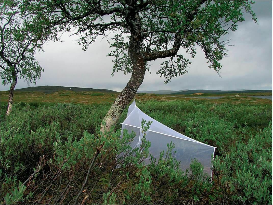
Fig. 1. The malaise trap by which the female of Gimnomera freyi sp. n. was collected on an alpine willow heath at the Muotkatunturi wilderness area in North Finland. Photo: Eerikki Rundgren.
